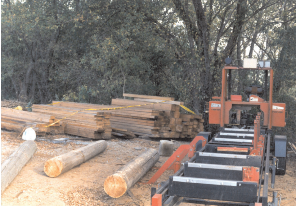
Western redcedar poles are sawn into various lumber dimensions on a portable sawmill. Photo by Kerry Burruss
